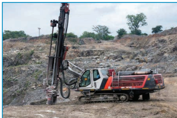
Modern Environment Friendly Hydro Static Drill Machine
